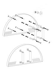
3. Install the door handles with 4 pcs of 1/4"\*15mm screws + insulation mat + flat washer + spring washer + 1/4" bolts. Don't place door on oven until your finish step.
