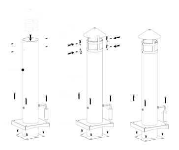
4. Install chimney cap with 4pcs of 5/32"\*10mm screws.
