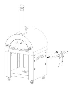
9. Install 3pcs of "L" short hooks and 1pc of long "L" hook with 8pcs of 1/4" \*15mm screws.
