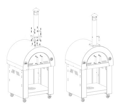
6. Install chimney with 4pcs of 1/4"\*15mm screws.
